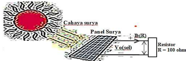
Gambar 7. Tegangan V_{O(sel)} mensuplai beban resistor R = 100 \Omega
