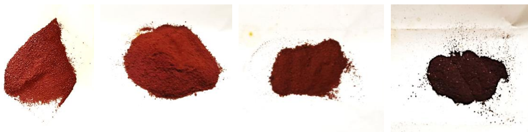
Gambar 2. Pigmen Besi Oksida hasil sintesis a). HCl 1 M+NaOH 4M, b). HCl 4M+NaOH 4M, c). HCl 1M+ \text{NH}_4\text{OH} 4M, dan d). HCl 4M+ \text{NH}_4\text{OH} 4M
