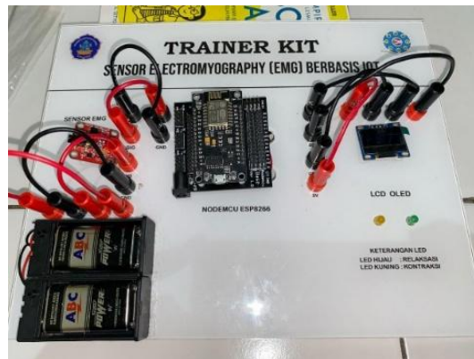
Gambar 8. Modul Electromyography (EMG)
