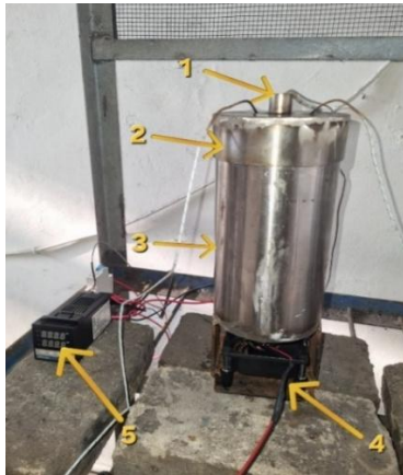
Gambar 3. Alat Thermal Energy Storage Keterangan bagian alat: 1.) Cartridge heater , 2.) Tutup tabung stainless steel , 3.) Tabung stainless steel , 4.) Kipas pendingin, 5.) Power control heater ( Temperature Thermostat REX C100 ).
